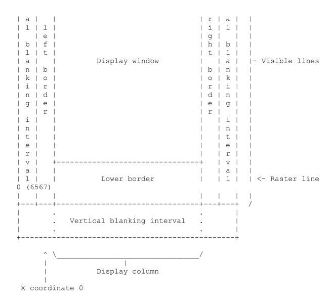
The height and width of the display window can each be set to two different values with the bits RSEL and CSEL in the registers \$d011 and \$d016:
