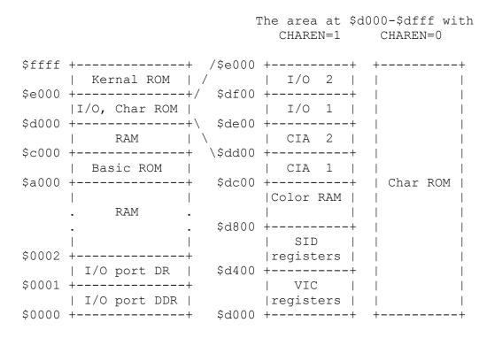
Basically, the 64KB main memory can be accessed in a linear fashion, but they are overlaid by ROM and register areas at several positions. A write access to a ROM area will store the byte in the RAM lying "under" the ROM. The 6510 I/O port is mapped to addresses \$0000 (for the data direction register) and \$0001 (for the data register).
