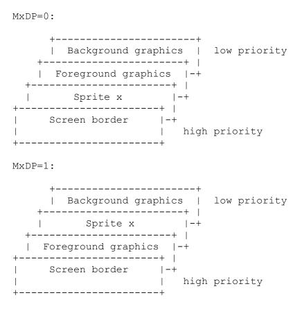
Of course, the graphics elements with lower priority than an overlayed sprite are visible where the sprite has a transparent pixel.
